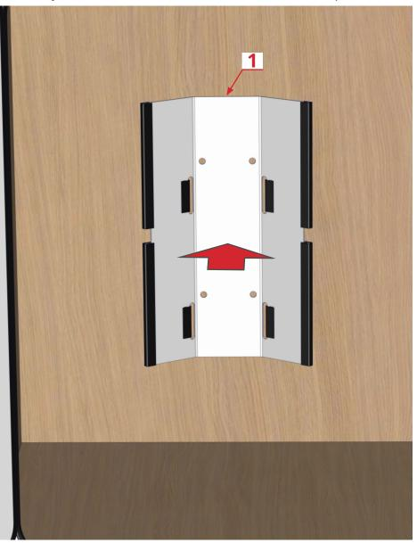
IMPORTANT- The front bracket should be raised from the floor so much that the notch on the bracket matches with the weld seam on the gas bottle!
