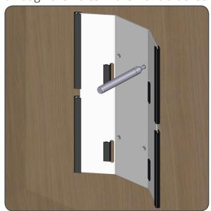
**Step 4-** Drill 4 holes using a 10mm drill bit.
