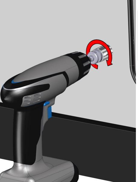
**Step 14-** Mark the 4 holes for the fixing screw + drill the holes using 5mm drill bit.
