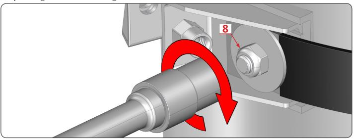
**Step 11-** Fix the buckles with the star handle screws by hand.
