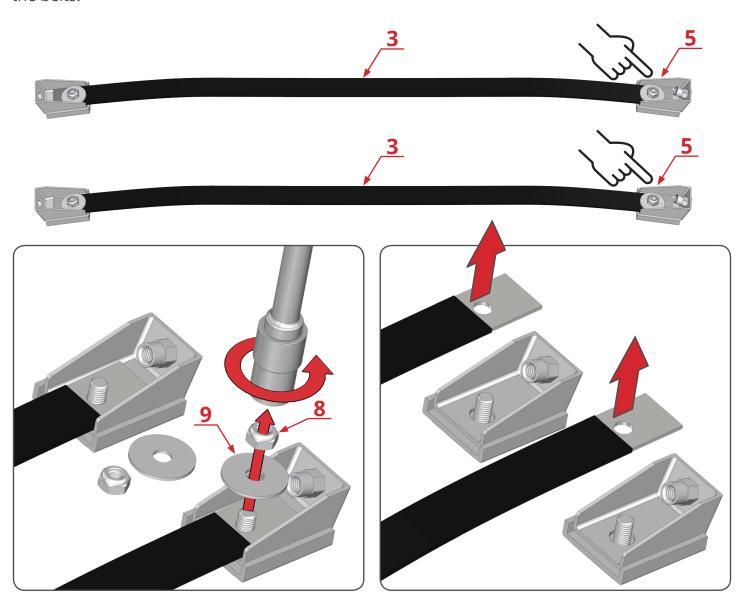
**Step 6-** Pass the both belts through the holes in the front bracket.
