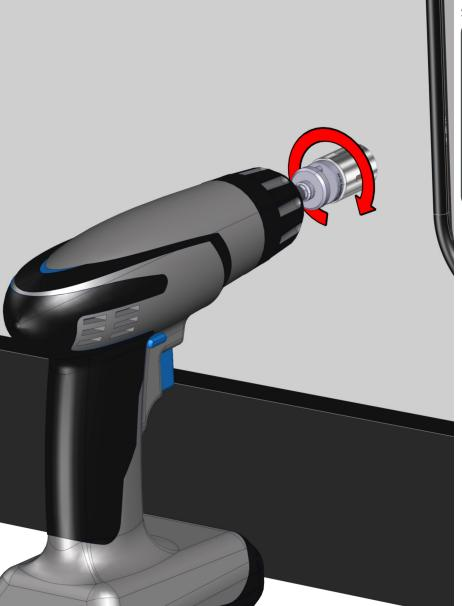
**Step 14-** Mark the 4 holes for the fixing screw + drill the holes using 5mm drill bit.
