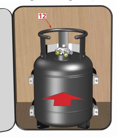
**Step 10-** Fix the buckles with the round-head bolts, lock washer and 16mm washer by hand.
