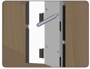
**Step 4-** Drill 4 holes using a 10mm drill bit.
