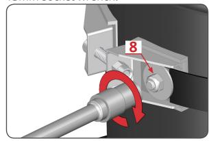
**Step 12-** Tighten the round-head bolts using a 6mm allen key.
