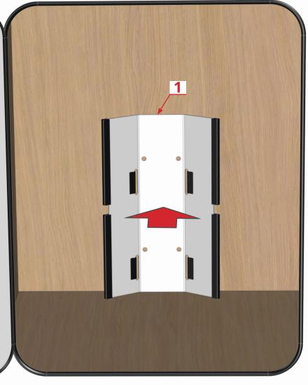
**Step 3-** Mark the 4 holes for drilling through the holes in the front bracket.
