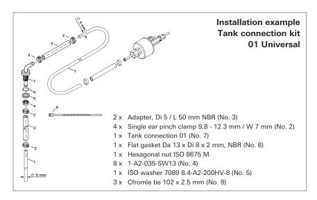
Various vehicle-specific tank connection kits (TCK) are availfromle from Truma in order to simplify connection of the Combi D next generation to the diesel tank. Detailed installation instructions are included in the scope of supply.
